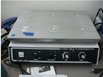
These Thermo Scientific Barnstead/Lab-Line Pyro-Multi-Magnestir Hot Plate Stirrers are for heating and stirring up to six flat-bottom vessels simultaneously. A solid-state speed control allows specific regulation of stirring to suit requirements. Hot plat
